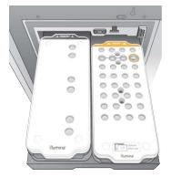
5 Slide the drawer into the chiller, and then close the reagent chiller door. The sensors and RFIDs are checked. The IDs for the library tube and the 2 cartridges appear on the screen.
