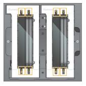
4 Select **Close Flow Cell Door**. The flow cell door closes, the sensors and RFID are checked, and the flow cell ID appears on the screen.
