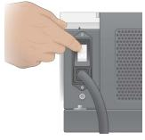
2 Wait until the power button on the right side of the instrument glows blue, and then press it.
