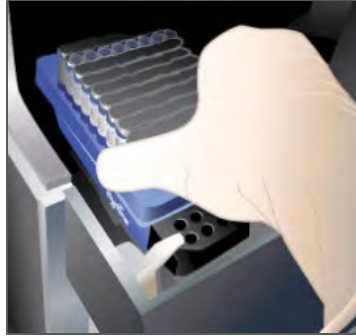
Figure 16 Position the Reagent Plate (showing a reagent plate for a High Output flow cell)
