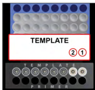
Figure 26 Tube Strip Orientation for HiSeq Rapid Flow Cell
