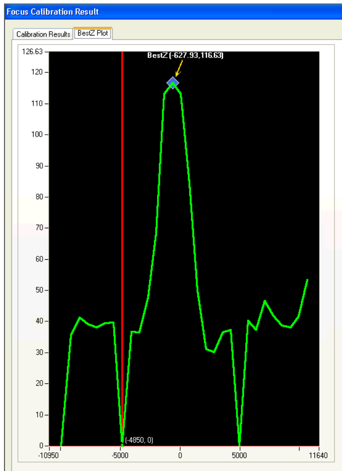
Figure 36 Focus Calibration Results, BestZ Plot Tab
