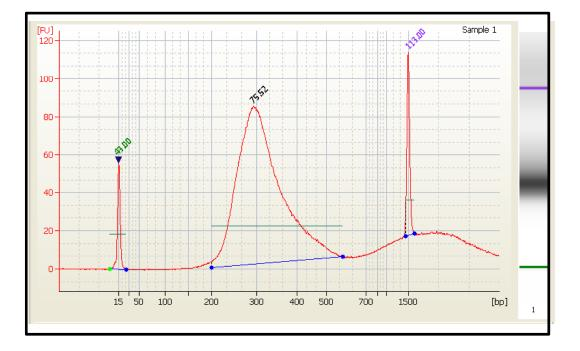
**Cause** : SPRI bead carryover from post-PCR clean-up step. Use a strong magnet for bead separation and pipette carefully during elution to avoid disturbing beads.
