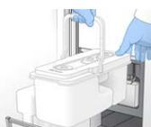
Unload consumables from the previous run and load consumables for the current run. Empty and reload the used reagent bottles.
